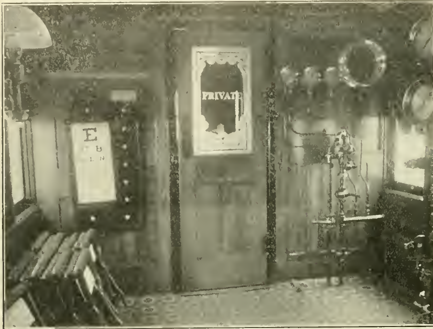
Fig. 3—TEXAS & PACIFIC RAILWAY AND INTERNATIONAL & GREAT NORTHERN R. R. AIR-BRAKE INSTRUCTION CAR—VIEW SHOWING BRAKE VALVE AND GAGES.
